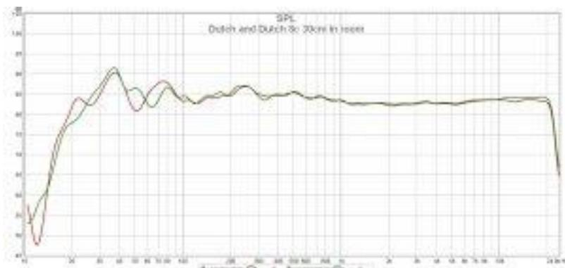
The room's standing waves are encroaching at low frequencies, but there is virtually no speaker boundary interference. The back of the 8c's are (L) 28 cm and (R) 38 cm away from the front wall. Optimizing this distance in the Active Room Matching user interface, for both left and right speakers, virtually eliminates any SBIR. These measures are with no PEQ's applied.
