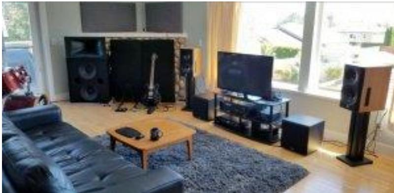
I pushed my large JBL speakers to the sides and set up the 8c's on my 24" sand filled, Monolith stands and placed the 8c's ~30cm from the front wall, as measured to the back center of the subwoofers. Vibrapods are used to isolate the speakers from the stands and the stands from the floor. I did not move the subs out of the way, but they were not hooked up for this evaluation.
