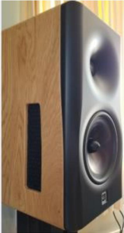
Each side of the cabinet has a cutout to the inside chamber of the midrange cabinet, which is used to passively control the midrange polar response to be a [cardioid pattern](#). This also controls [Speaker Boundary Interference Response](#) (SBIR). The idea is that the passive cardioid midrange (i.e. 100 Hz and up to the tweeter XO) outputs very little side and rear sound pressure so there is little to no speaker boundary interference.
