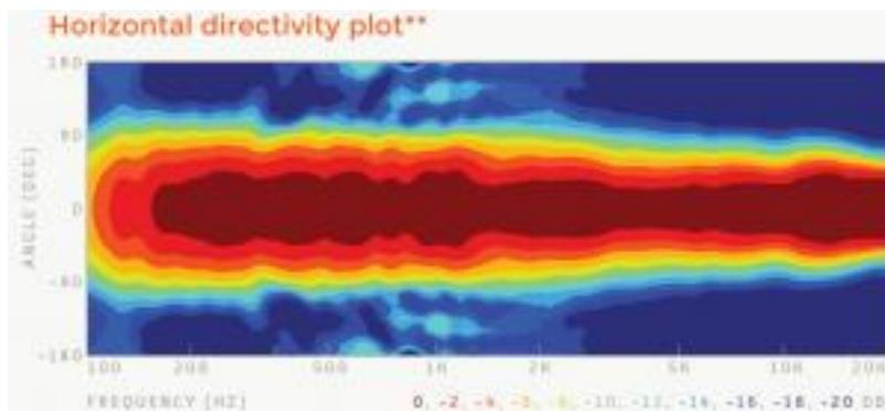
From 100 Hz on up, the on and off axis frequency response is incredibly accurate, best I have seen to date. The midrange driver is an 8” aluminum cone crossed over at 1250 Hz using a 4th order Linkwitz-Riley linear phase crossover to a 1” aluminum/magnesium alloy dome tweeter. Specs [here](#).
