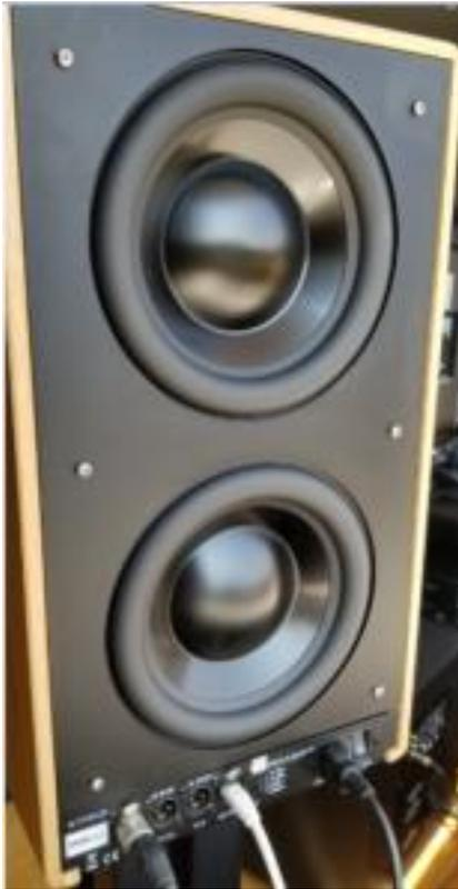
On the back of the loudspeaker are two 8" aluminum cone subwoofers operating from 100 Hz on down in a sealed cab. Yes, that's right, the dual subwoofers are built in. With their large linear max excursion design, these bad boys have an amazing amount of low frequency impact. That impact is further realized by being close to the front wall boundary, leveraging what is called the [Allison effect](#), named after the late [Roy Allison](#).
