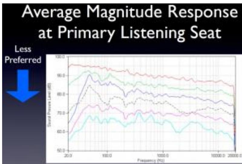
The top preference (red trace) is a flat, but tilted measured response. If 0 dB is 20 Hz, then it would be a straight line to -10 dB at 20 kHz. The “trained listeners” curve in Figure 14 in the Toole reference is similar.
