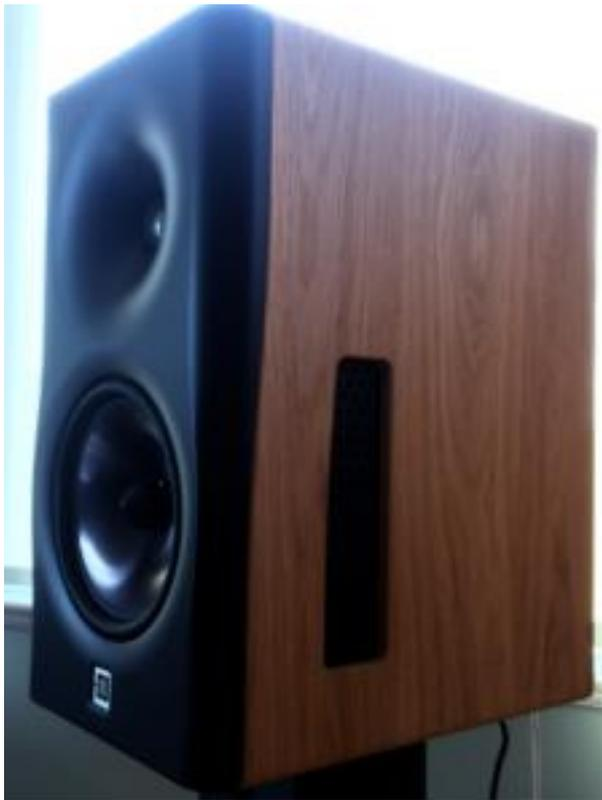
The [D&D 8c's](#) are the first loudspeakers to come into my room where I could achieve studio control room frequency response accuracy of 21 Hz to 20 kHz  $\pm 3$  dB at the listening position without any [external DSP](#).
