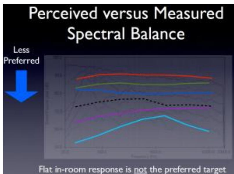
See how an objectively measured response of 20 Hz and straight line to -10 dB at 20 kHz is subjectively perceived as a neutral or flat response to our ears/brain (red trace overlaid in the above chart). Most participants in the study preferred a frequency response from 20 Hz with a straight line to -10 dB at 20 kHz. A measured “flat” in-room frequency response is not the preferred target, as it sounds too thin or lacking bass.
