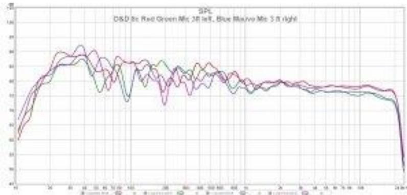
Impressive. Simply the HF level is a bit lower with very little high frequency response deviation over a six foot listening area. Virtually perfect off axis high frequency response from 1 kHz on up.
