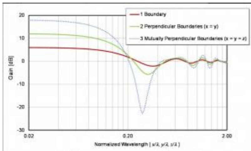
Even more low frequency room gain can be had using perpendicular boundaries, but at the expense of increased [speaker boundary interference response](#) (SBIR) above 100 Hz. In the linked article, scroll down to bookshelf loudspeaker to see a great example of SBIR.
