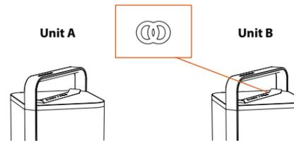
The pairing sequence between unit A and B will start. Both Twin buttons will start flashing blue and white every 2 seconds. Unit B will act as the Twin device.
