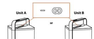
The blue LEDs on master and twin unit will turn white, indicating that Twin mode has been disabled on both units.
